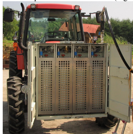
Fig. 1 The tractor equipped with a biogas unit
