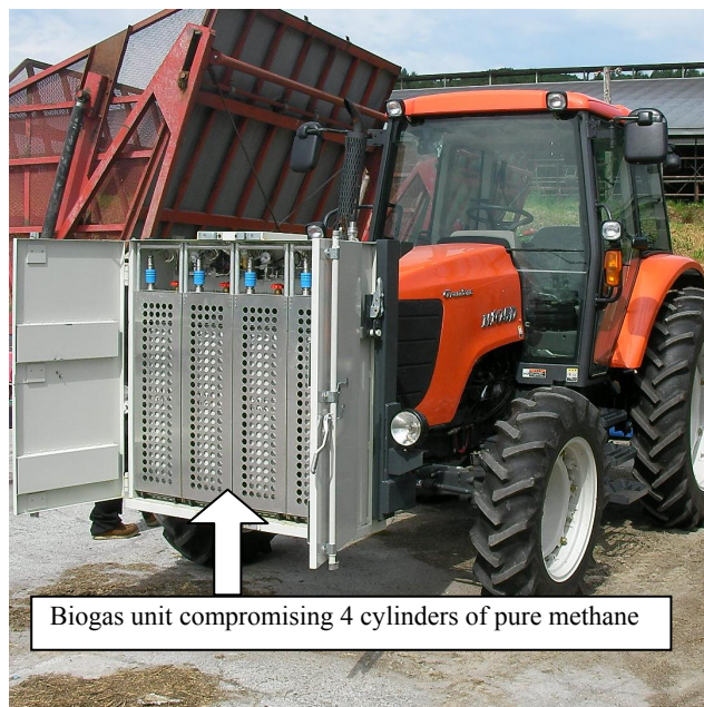
Fig. 1: the biogas tractor with its biogas unit opened to show the 4 cylinders of biogas
