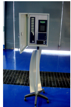
Fig. 5. Engine simulator manufactured to diagnose ECMs problems
