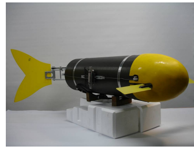
Figure 5: BAUV which has a variable-compliance caudal joint
