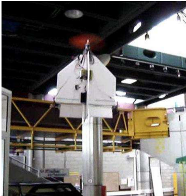
Fig. 7. The T-Plane UAV hovering autonomously.
