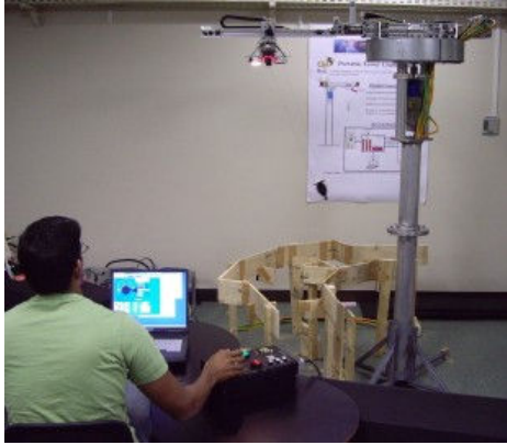
Fig. 6. Portable Tower Crane
