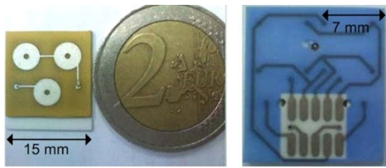
Figure 6 Planar MPA frontside (left) and backside (right)
