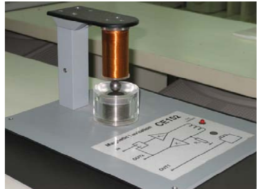
Fig. 3. The image of a practical experimental magnetic levitation system
