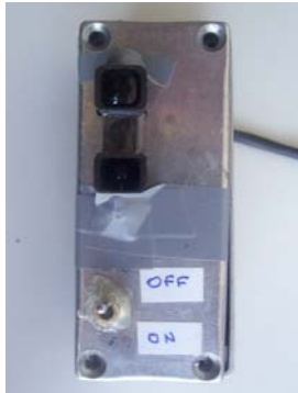
Fig. 4. Aluminium case containing the sensor and the battery supply.
