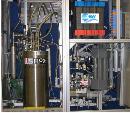
Fig. 5. Fuel cell-based power plant at ZSW Stuttgart, Germany
