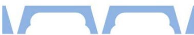
(d) The 2 nd cavities are etched by HF solution, and poly-silicon is removed by alkaline solution.
