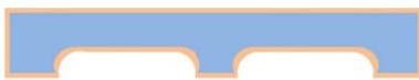
(b) The 1 st cavity is etched by HF solution, and poly-silicon is deposited.
