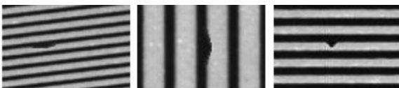
Fig. 2. (a) Deep wide protrusion, (b) shallow wide protrusion and (c) deep narrow protrusion
