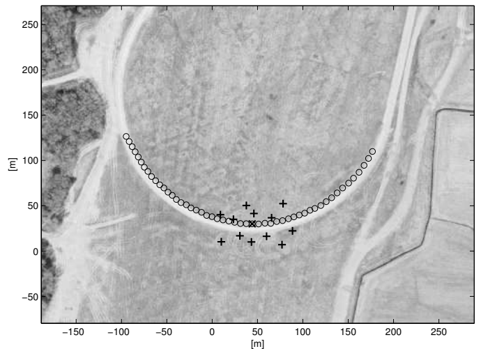
Figure 4. Sensor node locations and sample trajectory for motor cycle.
