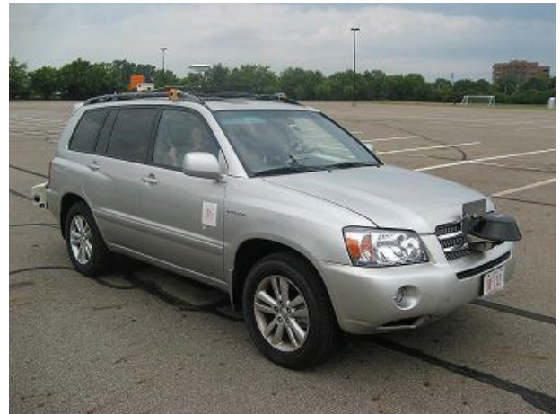
Fig. 2, OSU-ACT with front and rear looking LIDARs and GPS antenna visible.
