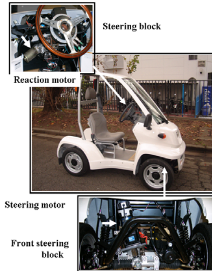
Fig. 7. Experimental vehicle with SBW system
