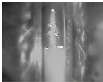
Fig.7. Edge Images. The white pixels are the strongest edges detected in each column
