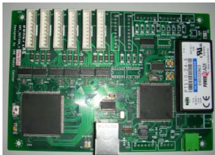
Fig. 5 Picture of small size 8-axis motion board
