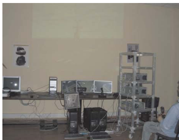
Fig. 1. The in-house developed network mission simulator allows real-time simulation across interoperable manned-unmanned fleets, and the mission control center.[25]
