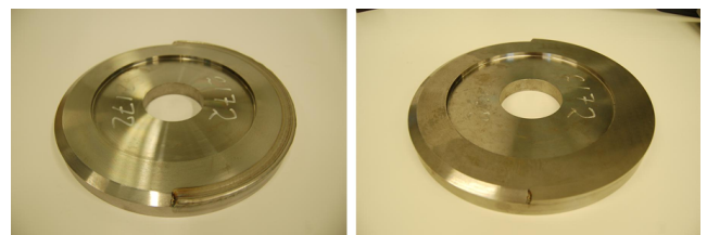
Fig. 4. Left: A circular mild steel plate with the original chamfered edge seen on the left half of the plate, and the deposited tool steel material on the right half. Right: The same plate with the new sharp edge, obtained after machining.
