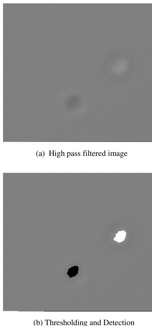
Fig. 2. Mura detection using high pass filtering based on average operation.
