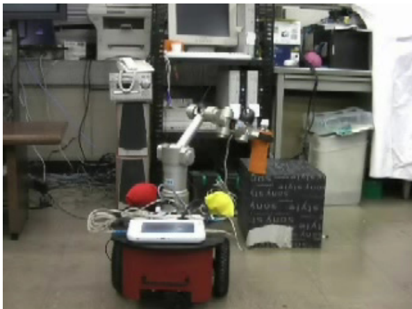
Fig 5.1: The robot arm is gripping a paper cup
