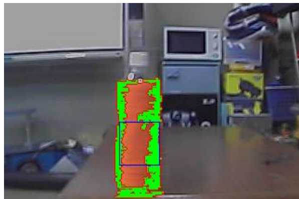
Fig 3.1: Tracking object's colour
