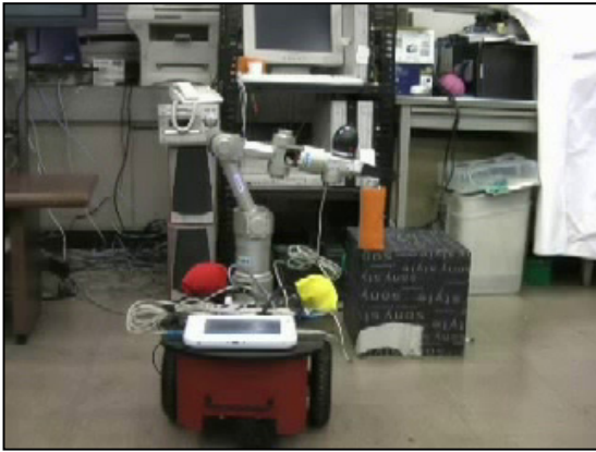
Fig 4.2: Six degree of freedom version arm
