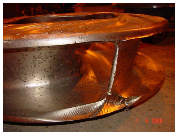
Fig. 9. A half worn out impeller of a final tailing pump at the Suncor oil sands plant.
