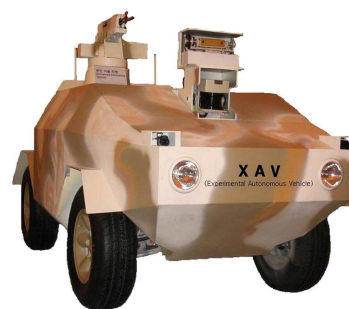
Fig. 1. UGV in consideration, its mass, momentum of inertia, length and width are 807 kg, 429.649 kgm 2 , 2.150 m, and 1.290 m, respectively.
