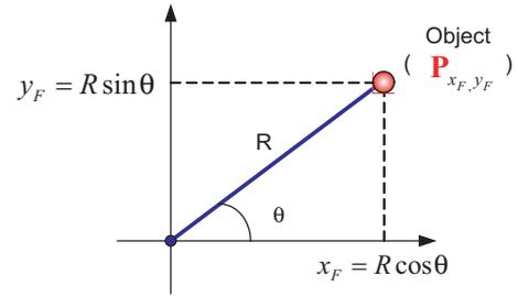
Fig. 2. Relationship between distance and angle for target object
