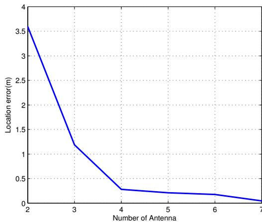
Fig. 5. Location error according to the number of antennas
