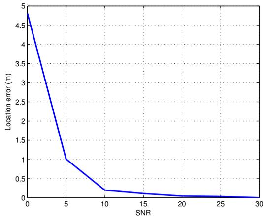
Fig. 4. Location error according to the SNR
