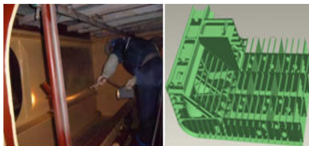
Fig. 1. The figure of Inner Double Hull Block
