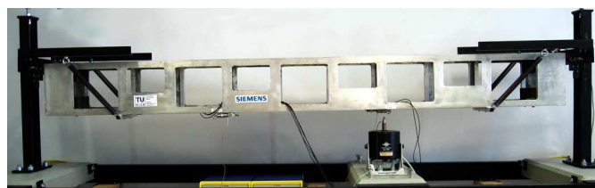
Fig. 1. Experimental setup of a scaled railway car body
