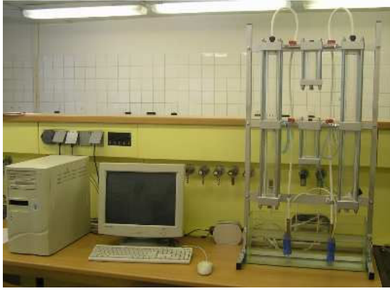
Figure 1. A front view of the quadruple tank system.
