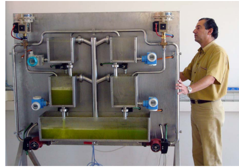
Fig. 1. Industrial Scale Model of 4 tanks used in the IUN.
