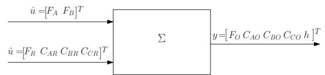
Fig. 6. System Representation of Reactor with Recycle (with controller)
