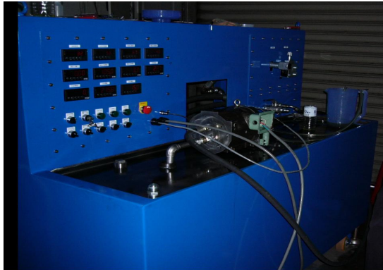
Fig. 11. Solid test for an electron-hydraulic pump of type EHP15-15
