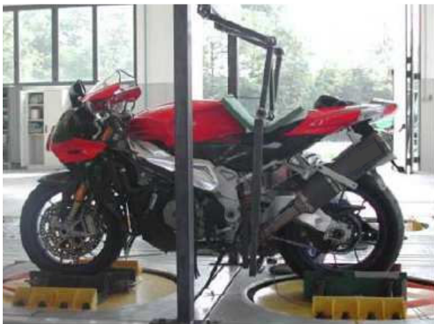
Fig.5. The MTS test rig at ISMA with a sustaining structure for two wheels testing.
