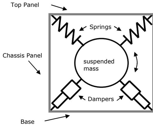
Fig.5. Scheme of the washing machine.
