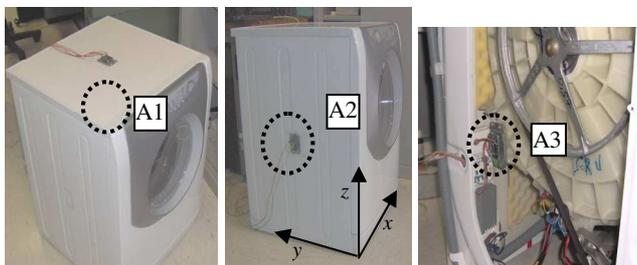
Fig.6. Sensor positioning. Top Panel (A1), Chassis Panel (A2), Drum (A3) accelerometers.
