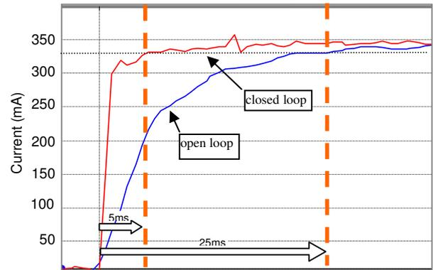
Fig.4. Time response to a step-like current command. Open and closed loop response.
