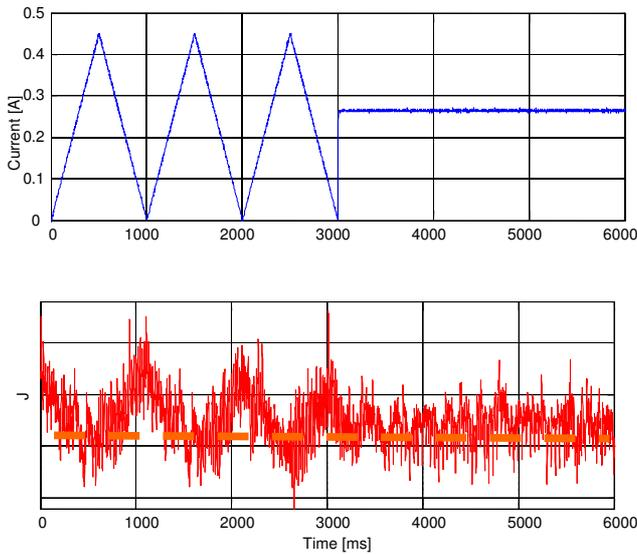
Fig.9. Adaptation strategy of the current in the time domain (1400rpm). Control signal (top) and performance index  $J$  (bottom - the scale is omitted for confidentiality reasons).
