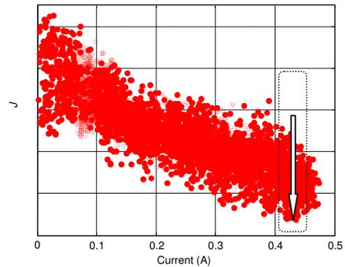
Fig.8. Performance index  $J$  with respect to the driving current. (1400 rpm)
