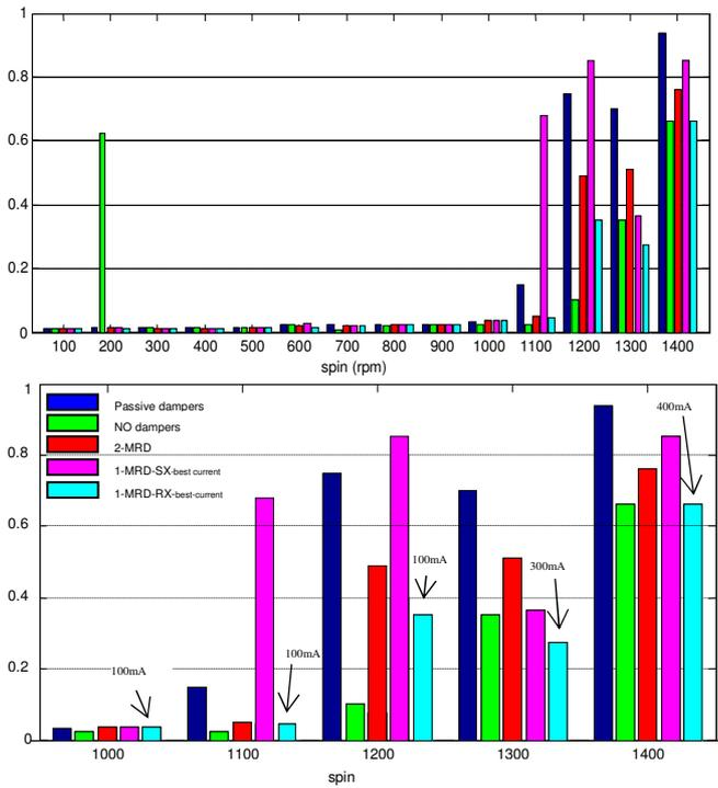
Fig.7. Performance index  $J_{vib}$  for different mounting configuration
