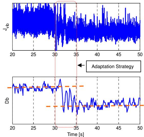
Fig.10. Experiment in anechoic chamber. Performance index of vibration level (top) and acoustic noise (bottom) during a 1400rpm adaptive control test. Both the scales are omitted for confidentiality reasons.
