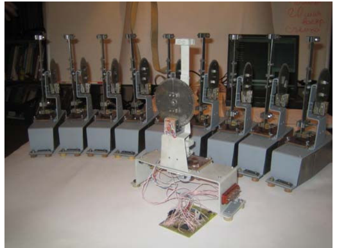
Fig. 8. The “Chain of Pendulums” mechatronic set-up (photo).
