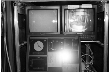
Fig. 2. Romeo ROV interface: pilot and coring monitoring camera images are shown in the monitors.
