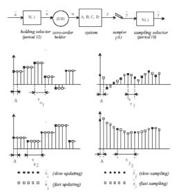
Figure 3. Multirate system mechanism
