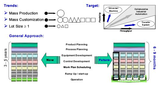
Fig 1. Production system engineering process - today and tomorrow
