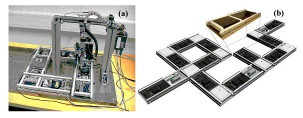
Fig. 6. (a) ABAS pilot installation in a micro-assembly cell (b) Actor-based transporter
