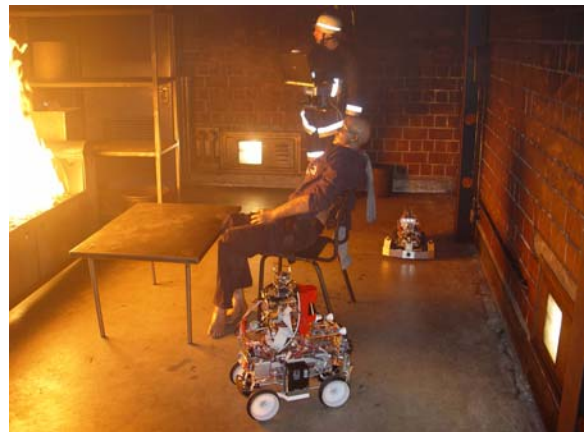
Fig.1: Robots guiding a firefighter during tests to persons to be rescued
