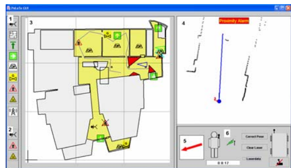
Fig. 5: Graphical User Interface for a rescuer in the emergency area, including similar information such as the supervisor's GUI and an personalized laser view according to his field of view, that visualizes the local map in front and the path to walk.
