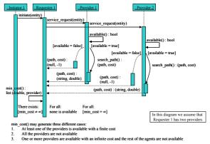
Figure 2: Part of the sequence diagram of the messaging protocol
