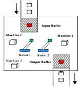
Figure 4: Illustrative Flexible Manufacturing Cell
