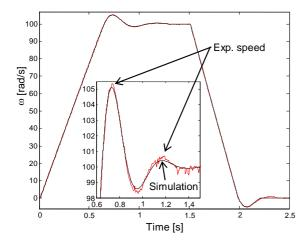
Fig. 8 Comparison of speed responses for  $J_{em}$ =10J,  $B_{em}$ =B and  $M_{z0em}$ =0.05 Nm
