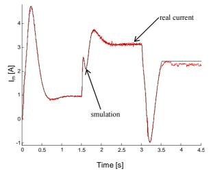
Fig. 12 Comparison of torque responses for  $J_{em}=3J$ ,  $C_t=0.1$  Nm.s/rad and zero dumping coefficient
