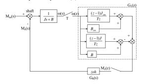
Fig. 2 Sampled inverse model system
