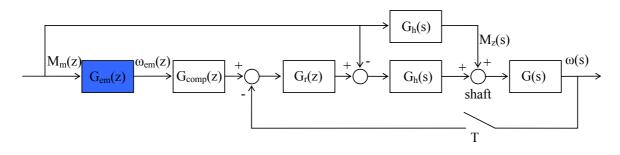
Fig. 3 Block system of "open loop" method
