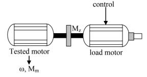
Fig. 5 General scheme of load emulator
