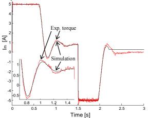
Fig. 9 Comparison of torque responses for  $J_{em}$ =10J,  $B_{em}$ =B and  $M_{z0em}$ =0.05 Nm
