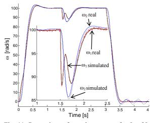
Fig. 11 Comparison of speed responses for  $J_{em}=3J$ ,  $C_t=0.1$  Nm.s/rad and zero dumping coefficient
