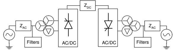
Fig. 1. High Voltage DC scheme
