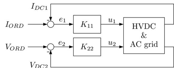
Fig. 2. Control configuration for HVDC transmission link
