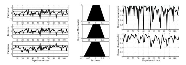
Fig. 8. Detection of operating conditions with LE models: fuzziness and limits of fuzziness for three equations and the resulting degrees of membership for each data point (upper curve) and a moving average (lower curve).
