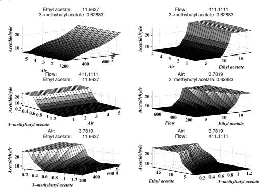
Fig. 7. Model surfaces of a five variable LE model on a normal operating point.
