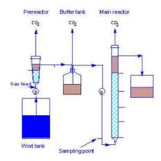
Fig. 2. Pilot scale continuous fermentation system.
