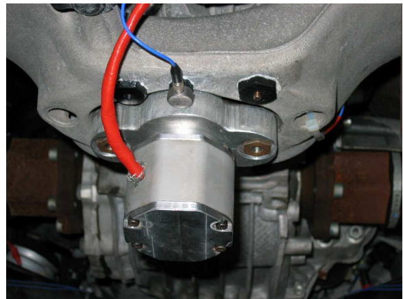
Fig. 2. Location of actuator and sensor in a test vehicle.
