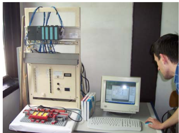
Fig. II. One working centre with PLC SIEMATIC S7-300, Simulation station, simulating process and computer with software STEP 7
