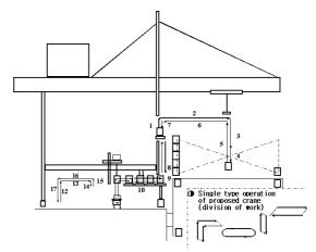
Fig. 4. An Operation process of new type crane system. (single cycle)
