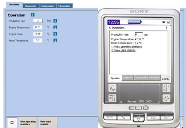
Fig. 6 Useware prototypes for Web client and PDA.
