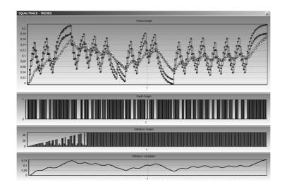
Fig. 4. SQualTrack fault detection. Case 2: J-bigger. Upper graph shows envelopes of measurement and simulation. Following graph shows bars with 1 when a fault is detected. Next graph indicates last window length applied at the specific time. Lower graph shows the analyzed measurement.
