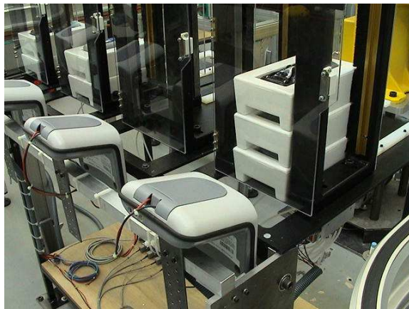
Fig. 8. Work in process buffer for packing robot.
