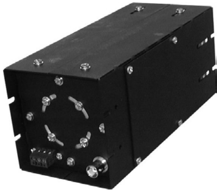
Fig.3. Embedded system with CCD camera prepared for installation in TERADYNE test machine.
