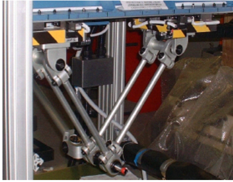
Fig. 1 Morpheum: reconfigurable parallel kinematics robot with four d.o.f.
