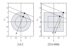
Fig. 2. The input that minimizes  $\dot{V}(x,u)$  in  $\bar{U}'_{k}$
